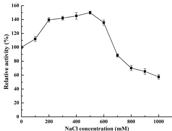
**Fig. 6** Effect of NaCl on the activity of LacHa. The activity was measured in 50 mM  $\text{Na}_2\text{HPO}_4\text{-KH}_2\text{PO}_4$  buffer at pH 7.5, supplemented with 100  $\mu\text{M}$   $\text{CuSO}_4$ , at 45 °C with 100  $\mu\text{M}$  syringaldazine as substrate
