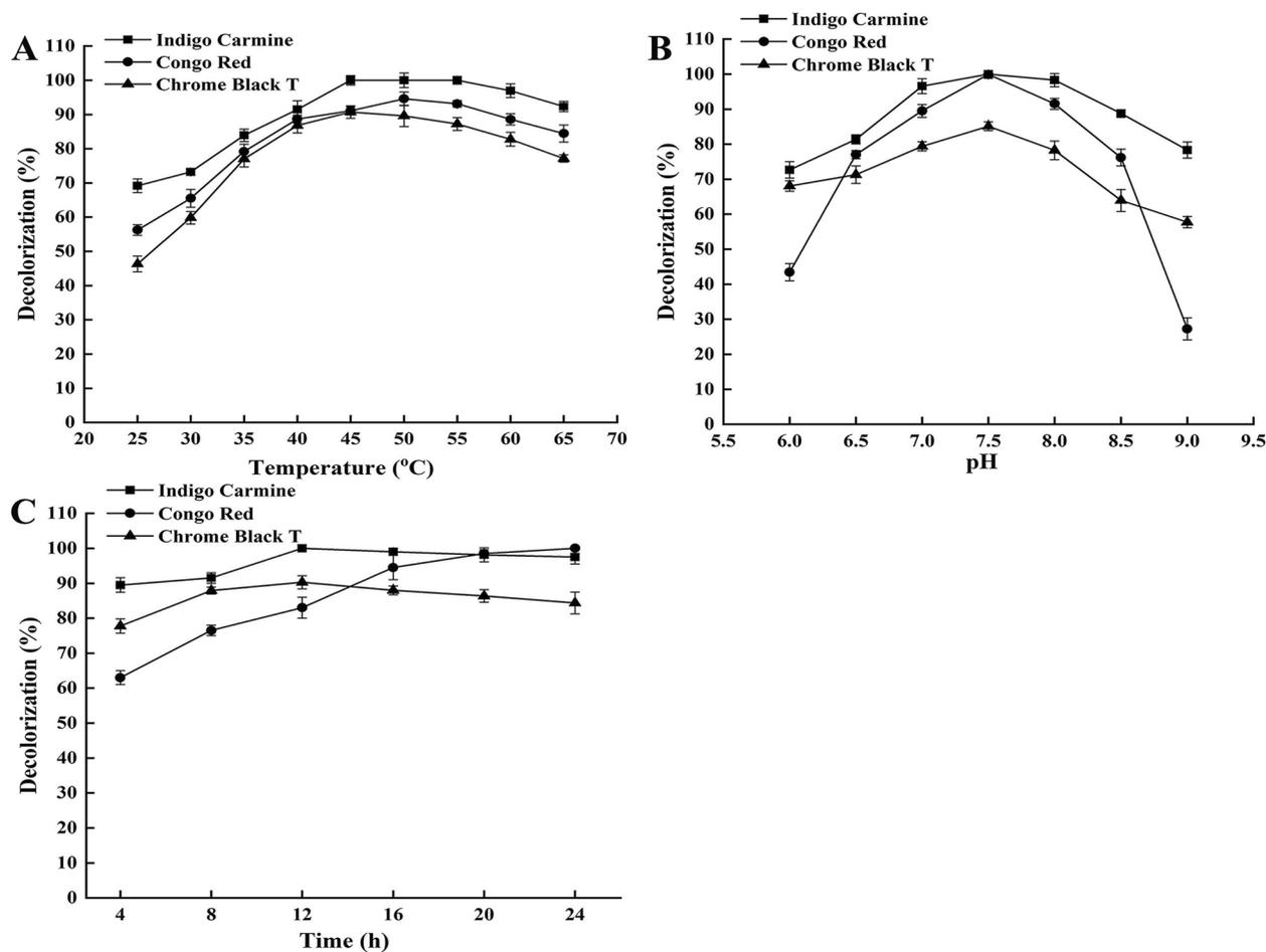
**Fig. 7** Effects of temperature (A), pH (B), time (C) on dye decolorization of LacHa. The values and standard deviations are calculated based on three independent experiments
