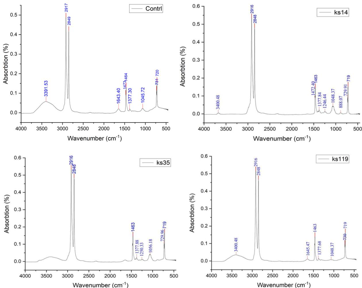
**Fig. 4** FT-IR spectra of polyethylene sheet treated with bacterial inoculum and the control incubated at 35 °C for 60 days. Peak at 1643.78  $\text{cm}^{-1}$  which represent C=C stretch of alkenes disappeared in all bacterial-treated LDPE film except KS 119-treated film. New peaks at 1250.9  $\text{cm}^{-1}$  and 1246.44  $\text{cm}^{-1}$  attribute to C–O stretch of ester's group
