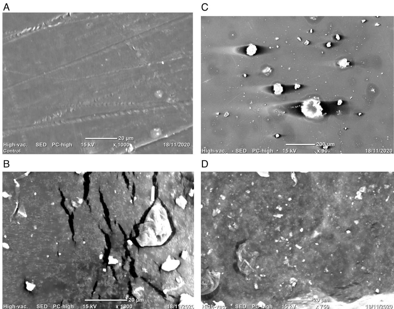
**Fig. 3** Scanning electron micrograph of LDPE films after 60-day incubation with bacterial isolates showing surface disruption, holes, and wrinkles on the surface. **A** Control, **B** LDPE film after treatment with KS14, **C** LDPE film after treatment with KS119, and **D** LDPE film after treatment with KS35
